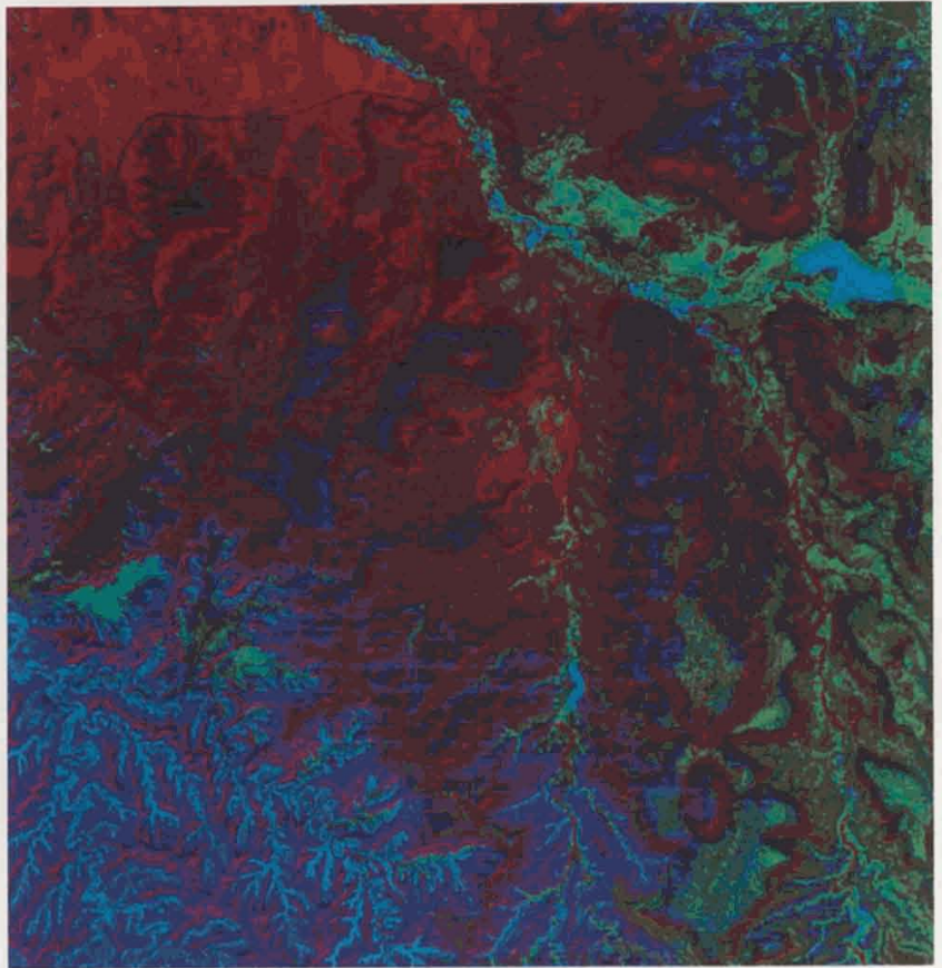
Landcover Classification: The image above shows a portion of Davis Canyon, Utah, after six spectral bands of TMS data were digitally ratioed in order to clearly delineate varieties of rock formations and vegetation. Sandstones, siltstones, and shales appear in several shades of blue, green, and purple, respectively; windblown sands appear red; and sage and salt-cedar concentrations appear light blue. The data for this image were acquired for a Department of Energy geologic mapping project.
