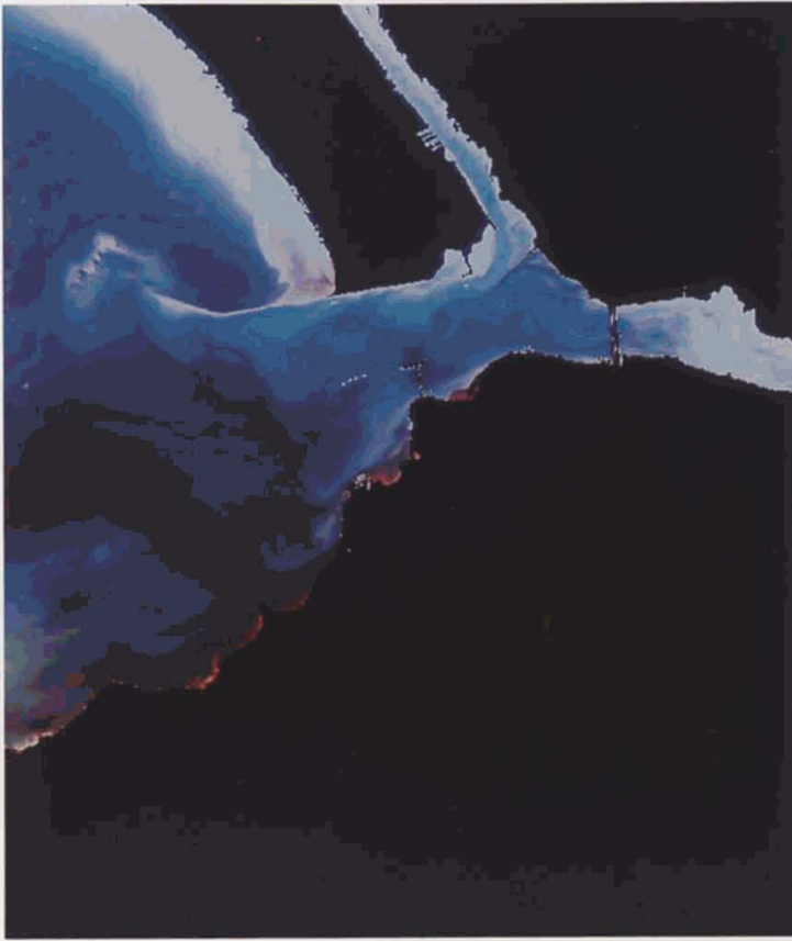
Water Enhancement and Color Infrared Imaging: These two images illustrate multiple applications of a single TMS data set. The water-enhancement image (left) uses TMS channels 1, 2, and 3 to show the transport patterns and distribution of suspended sediments as clear ocean water mixes with the outfall of the Sacramento River. The color infrared image (right) uses visible infrared waveband data to point up vegetation and land use features. Color infrared images are generally very useful for distinguishing between basic land cover types (vegetation, water, bare earth, and urban settlement) as well as for distinguishing type, maturity, or condition of specified areas of vegetation. The data for the images above were acquired for a NASA Ames study of estuary processes.
