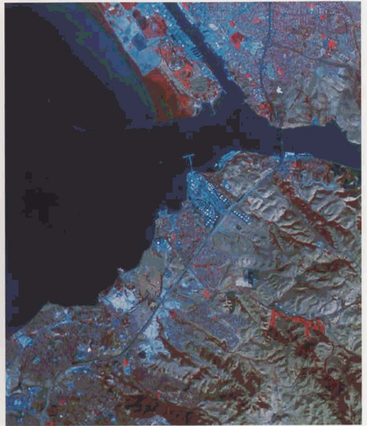
Water Enhancement and Color Infrared Imaging: These two images illustrate multiple applications of a single TMS data set. The water-enhancement image (left) uses TMS channels 1, 2, and 3 to show the transport patterns and distribution of suspended sediments as clear ocean water mixes with the outfall of the Sacramento River. The color infrared image (right) uses visible infrared waveband data to point up vegetation and land use features. Color infrared images are generally very useful for distinguishing between basic land cover types (vegetation, water, bare earth, and urban settlement) as well as for distinguishing type, maturity, or condition of specified areas of vegetation. The data for the images above were acquired for a NASA Ames study of estuary processes.
