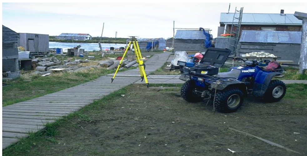
FIGURE 4. PHOTO ID GCP, RURAL ALASKA (COURTESY AERO-METRIC AK)
